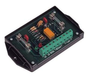
customer, but meter potentials are only on one service. To insure that the meter is always energized and measuring energy use, the APU-1x switches from the primary source to the auxiliary source if the primary source is lost.
