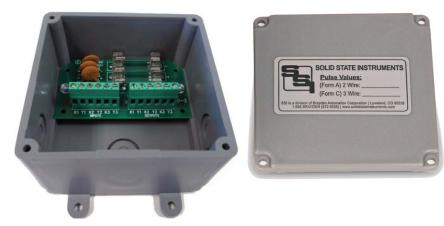
The CID-3's mounting configurations incorporates four knockouts for  $\frac{1}{2}$ " electrical conduit which can be used in a wide range of connection schemes to the electric meter's enclosure.
