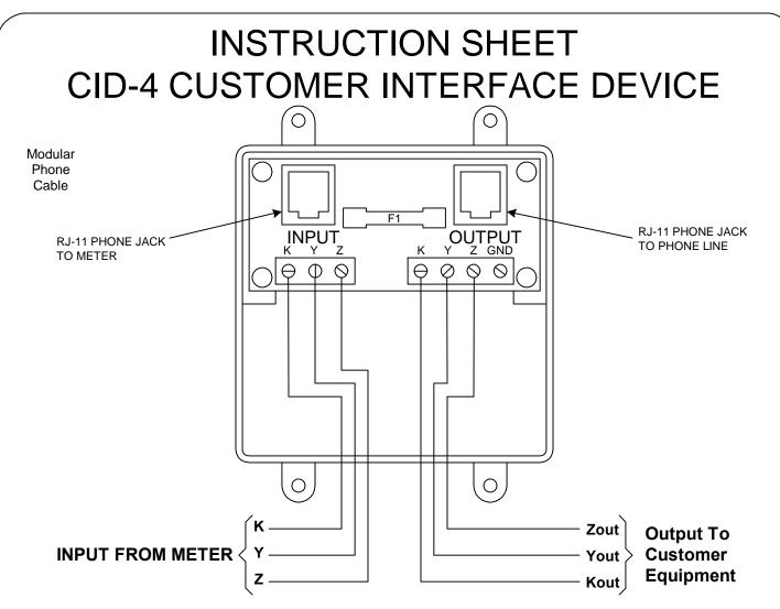
**MOUNTING POSITION** - The CID-4 can be mounted in any position. Use the knockouts on the back and sides to nipple the CID-4 onto the meter enclosure.
