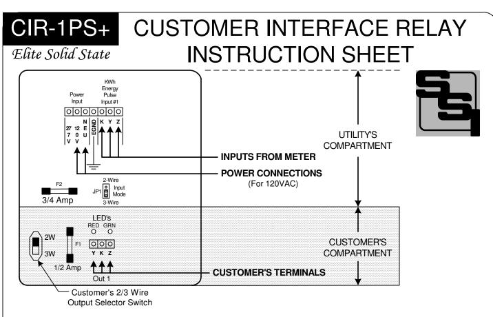
**MOUNTING POSITION** - The CIR-1PS+ may be mounted in any position.
