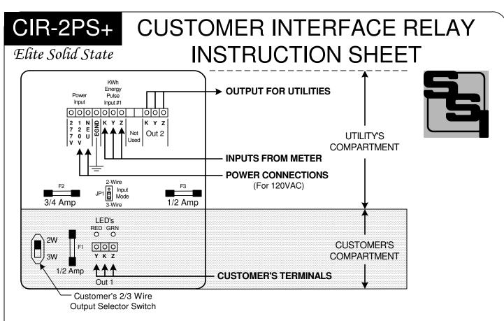
MOUNTING POSITION - The CIR-2PS+ may be mounted in any position.
