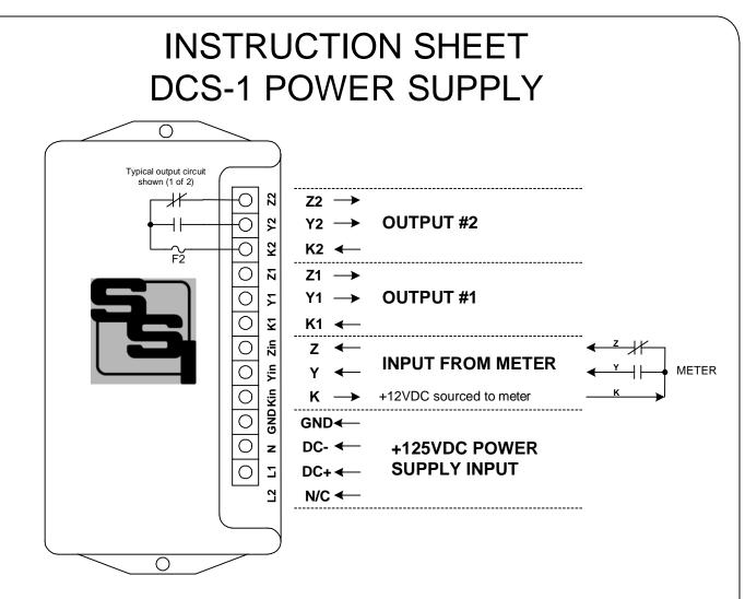
**<u>SUMMARY</u>** - This addendum accompanies any SSI Pulse Isolation Relay is equipped with the DCS-1 Power Supply option. This option allows you to power your relay from a 1+25VDC voltage source.
