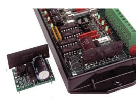
the DCS-1 supplies the relay's power supply requirements as well as providing a wetting voltage to the meter.
