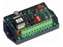
a single jumper shunt mounted on the relay's board and is easily adjustable by hand or with a set of needle nose pliers. The DPR-1 counts the input pulses for division only when a correct and valid sequence of pulses occur. Bright yellow and green LED lamps indicate the input and output status of the system at all times thus allowing a rapid visual check-out of the system's performance without requiring any additional test equipment.
