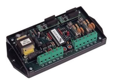
adjustable with a small screwdriver. The DPR-22PS microcontroller checks the input pulses for the correct sequence and timing, and counts the input pulses for division only when a correct and valid sequence of pulses occur, thus assuring a high degree of noise rejection. Two sets of bright red and green LED lamps indicate the input and output status of the system at all times thus allowing a rapid visual check-out of the system's performance without requiring any additional test equipment.
