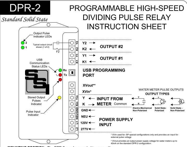
MOUNTING POSITION - The DPR-2 may be mounted in any position.
