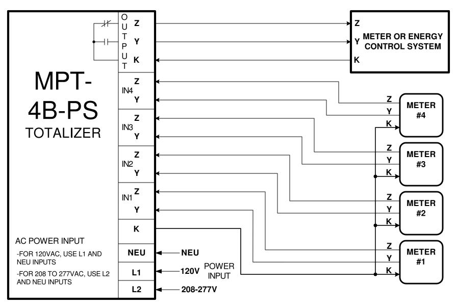
NOTE: A Sense Voltage of +13VDC is applied to the meters via the "Y" or "Z" leads from the MPT-4B-PS. The "K" lead is the common return.
