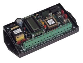
recorder applications, and supervisory control systems (SCADA) interfaces. The MPT-4B-PS pulse totalizer may also be used as a pulse value translator if it is desirable to translate odd pulse values such as 0.1234 KWH/pulse to an even value, 0.5000 KWH/pulse. The pulse inputs of the MPT-4B-PS are configured as four sets of Y & Z input terminals with a common "K" input terminal.
