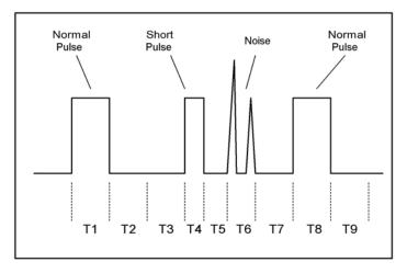
power systems are less then one cycle long, we recommend that the minimum setting be 30 milliseconds. This still allows a pulse input rate to the MPT-8B of 33 pulses per second, a rate much higher than usually experienced. The absolute minimum setting that the MPT-8B will accept is 10 milliseconds. The maximum time is 250 milliseconds. Entry is in 10 millisecond increments. The entry process is the same as that used with the meter input values.
