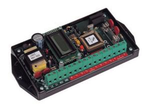
tions, and supervisory control systems (SCADA) interfaces. The MPT-8B pulse totalizer may also be used as a pulse value translator if it is desirable to translate odd pulse values such as 0.1234 KWH/pulse to an even value, 0.5000 KWH/pulse. The pulse inputs of the MPT-8B are configured as eight sets of Y input terminals with a common "K" input terminal.
