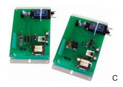
configuration selection. This system makes it possible to quickly implement an optical pulse link with minimal effort and includes all power supplies, wetting voltages, isolation relays and connectors.
