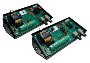
selection. This system makes it possible to quickly implement an optical pulse link with minimal effort and includes all power supplies, wetting voltages, isolation relays and connectors.
