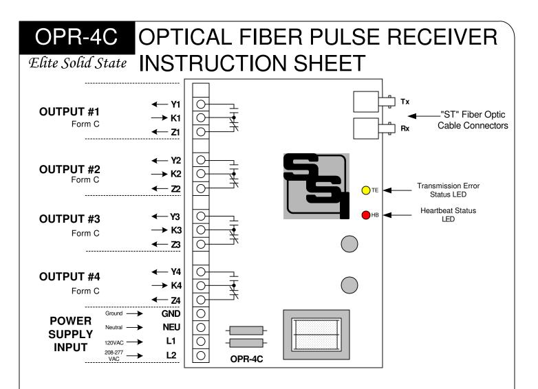
**MOUNTING POSITION** - The OPR-4C may be mounted in any position.
