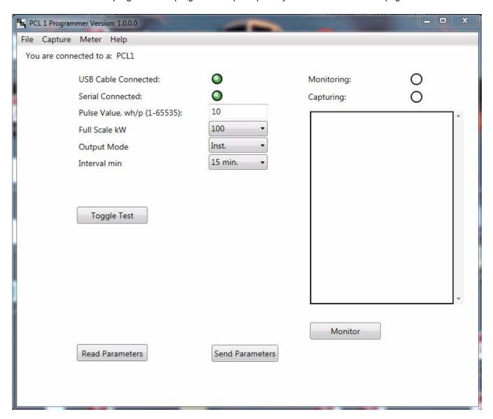
To READ the parameters currently stored in memory, click on <Read Parameters>. The PCL-1 Programmer will return the actual values of each parameter currently stored in EEPROM memory.
