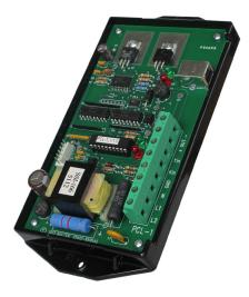
current level between 4mA and 20mA. For example, suppose you have the full scale output of the PCL-1 configured for 500kW. If a current demand of 250kW is calculated, the output would be adjusted to 12mA, the 50% midpoint between 4 and 20mA.
