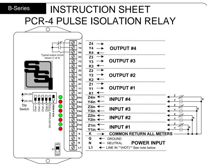
MOUNTING POSITION - The PCR-4 may be mounted in any position since it uses solid state relays.
