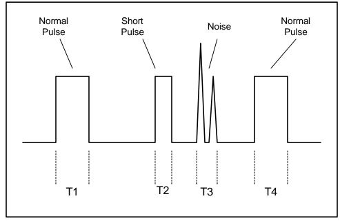
the time the input pulse is present. If the input pulse is present for less than the specified time (in milliseconds) as determined by the position of jumpers JP4 and JP5, it is assumed to be noise. An input equal or longer in duration than the specified time is classified as a valid input and an output will occur. In the illustration to the left.
