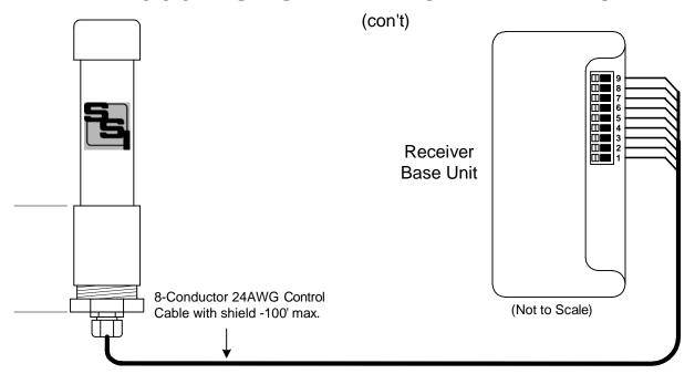
POWER INPUT - The PRR-900 receives its power supply from the PRR-2 Receiver Base unit.
