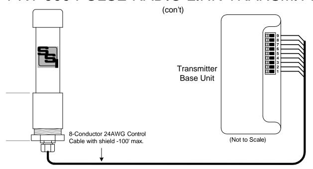
POWER INPUT - The PRT-900 receives its power supply from the PRT-2 Transmitter Base unit.
