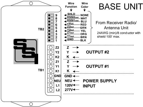
**GENERAL -** The PRR-2 serves as a base unit and termination point for the PRR-900 916.25 MHz radio receiver/antenna unit. It contains a power supply, output relays and all connection points for power and the radio receiver/antenna unit.
