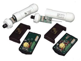
trenching or other costly methods of getting wires strung between the two devices. The PRL-900 Wireless Pulse Link system consists of a PRT-900 Transmitter and a PRR-900 Receiver. The system operates at 916MHz and allows unlicensed operation by the user. The PRL-900 will transmit pulses up to 1000 feet in a line-of-sight configuration. Longer distances may be possible with greater elevation above the ground.
