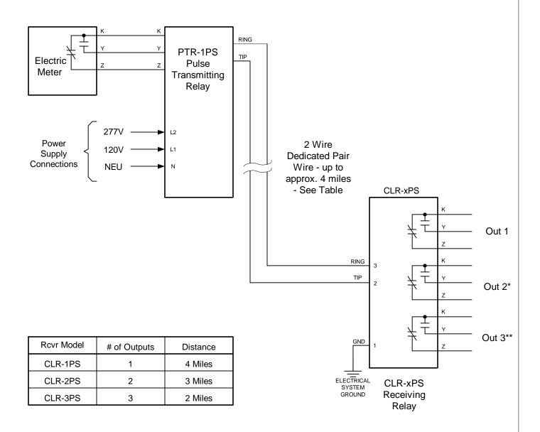
Operation: The PTR-1PS contains a +/-15 to 36VDC current loop for long distance pulse transmission and uses a dedicated pair of wires. As the PTR-1PS' KYZ input alternates from one closure to another, the current loop polarity reverses causing all output relays to switch in the CLR-x Receiving Relay. Maximum distance of transmission decreases with the increased number of outputs on the receiving relay. Maximum distance will also increase as wire size increases.
