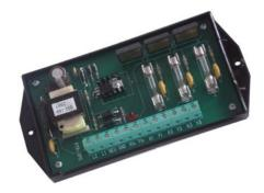
2PS is available in 1, 2, and 3 Form A outputs (K & Y). Its current loop design will adjust the output voltage to overcome and compensate for the resistance of the wire loop.
