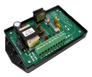
The RPR-1PS relay is designed to filter noise and transients from its input to prevent any false pulses at its output. Bright red and green LED indicators display the system's status at all times, thus allowing a rapid visual check of the system's performance without requiring any additional test equipment.
