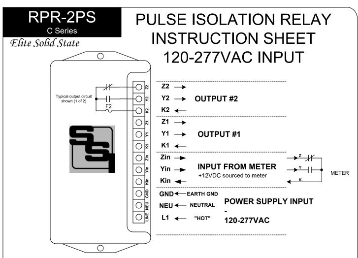
**MOUNTING POSITION** - The RPR-2PS contains solid state relays and can be mounted in any position.
