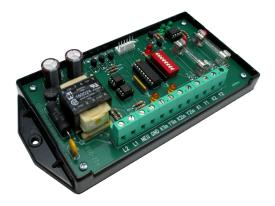
is switched from its "pulled up" state to ground (K) for at least a minimum pulse time. Four input filter times are field-selectable: 50 microseconds, .5, 5 or 20 milliseconds.
