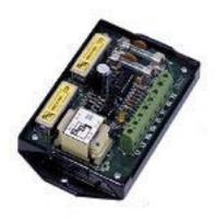
If Badger's RTR water meter provides an open-collector transistor output to interface to Badger's remote meter reading equipment, the RTR-2 relay is inserted in the two conductor cable between the RTR meter and the remote equipment. The RTR-2 provides a replicated signal to the remote equipment, and a separate isolated Form A contact closure for use with customer-owned monitoring equipment.
