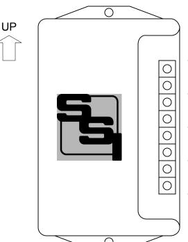
For Badger Record-All "RTR" Water Meters, Hersey ER-2 Water Meters and other Electric, Water & Gas Meters with open collector transistor outputs.
