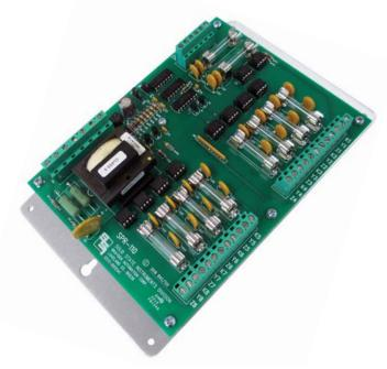
and is "pulled up." "Kin" is the common return. The SPR-110 may be used with meters having electro-mechanical output contacts (relays), or high or low voltage semiconductor outputs.
