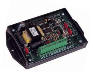
may be used with meters having high or low voltage semiconductor outputs, or electro-mechanical output contacts (relays).
