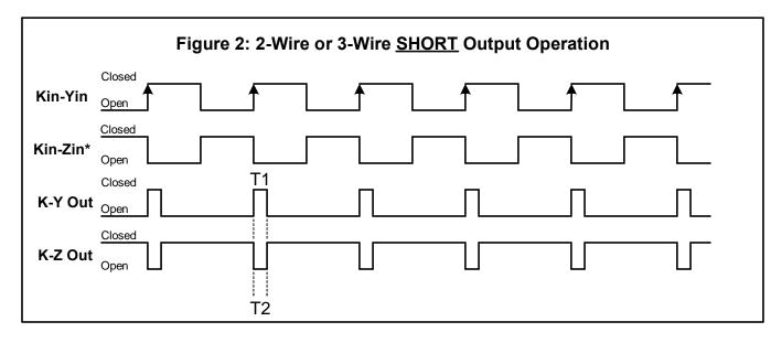
If the input pulse rate is greater than 9 pulses per second, it is recommended that the LONG pulse output mode be used. Contact the factory for technical support at (888)272-9336.
