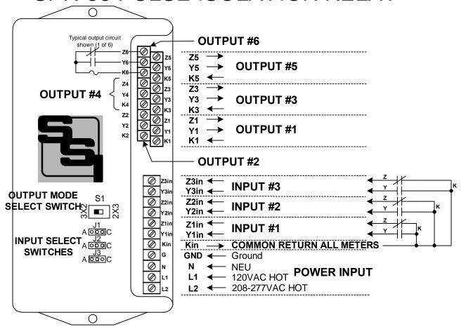
**MOUNTING POSITION** - The SPR-36 may be mounted in <u>any</u> position since it uses solid state relays.
