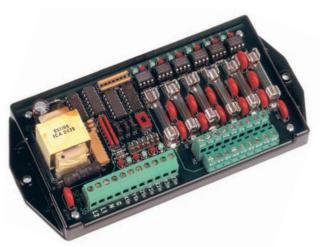
The SPR-36 operates over the standard SSI wide voltage range. The SPR-36 has a built-in low voltage transformer-isolated power supply generating a +13VDC sense voltage. The sense voltage is sent to each meter's Y and Z terminals from the SPR-36's Yin and Zin input terminals, returning to the Kin terminal, the common return for all meters. Since all meters supplying pulses to the SPR-36 have a common reference, a number of flexible input configurations can be wired.
