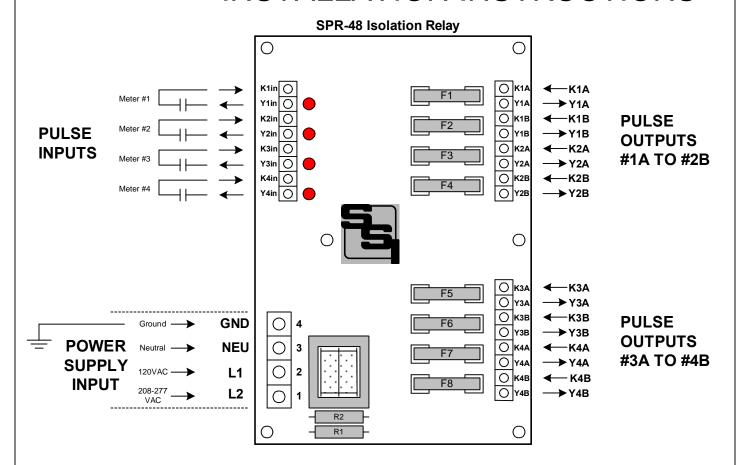
**MOUNTING POSITION** - The SPR-48 may be mounted in any position.
