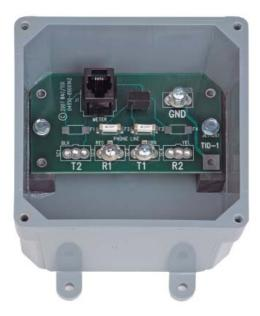
provides transient voltage surge suppression to protect the meter's modem from lightning or other electrical disturbances that may affect the telephone line inside the home or business.
