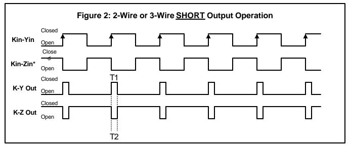
If the input pulse rate is greater than 9 pulses per second or if pulses of 100mS are too short for the receiving equipment, it is recommend that the <u>LONG</u> pulse output mode be used. Contact the factory for technical support at (888)272-9336.
