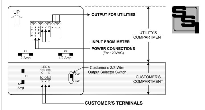
**MOUNTING POSITION -** Because the CIR-2A contains mercury-wetted relays, it must be mounted in a vertical position to operate correctly.
