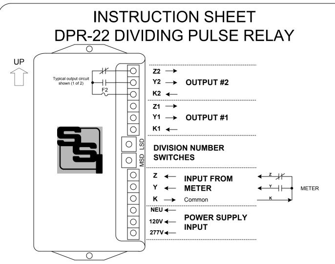
**MOUNTING POSITION -** Because the DPR-22 contains mercury-wetted relays, it must be mounted in a vertical position to operate correctly.
