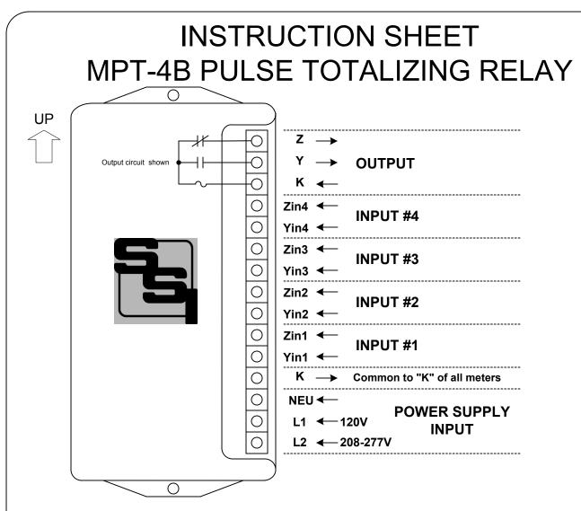
**MOUNTING POSITION -** Because the MPT-4B contains a mercury-wetted relay, it must be mounted in a vertical position to operate correctly.
