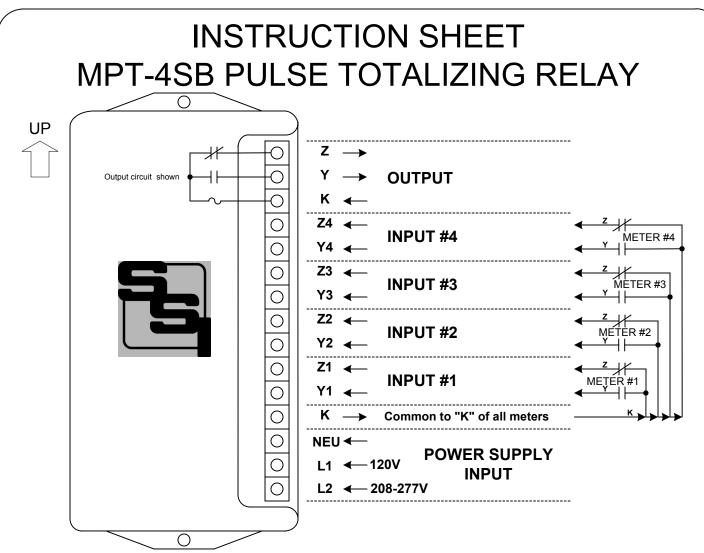
**MOUNTING POSITION -** Because the MPT-4SB contains a mercury-wetted relay, it must be mounted in a vertical position to operate correctly.
