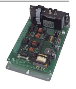
Bright red and green LEDs are included on the OPR-1 to monitor the output status. The dry contact output features a 1/4 amp solid-state relay for a no- bounce contact with internal MOV transient suppression circuitry to eliminate contact noise. Rapid pulse rates in excess of 20 pulses per second are possible.
