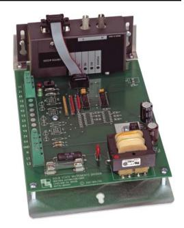
receiver where the pulse information is validated and implemented into the correct pulse state. An OPT-1 transmitter requires an OPR-1 receiver.
