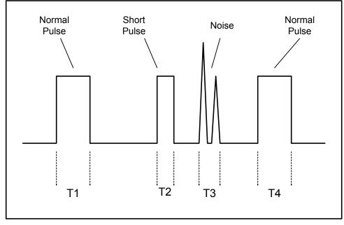
by measuring the time an input voltage is present. If the input voltage is present for less than 20 to 25 milliseconds. it is assumed to be noise. An input of longer duration is classified as a valid input and an output will occur. In the illustration to the left, the normal pulses with time durations of T1 and T4 will cause an output. The short pulse of time duration
