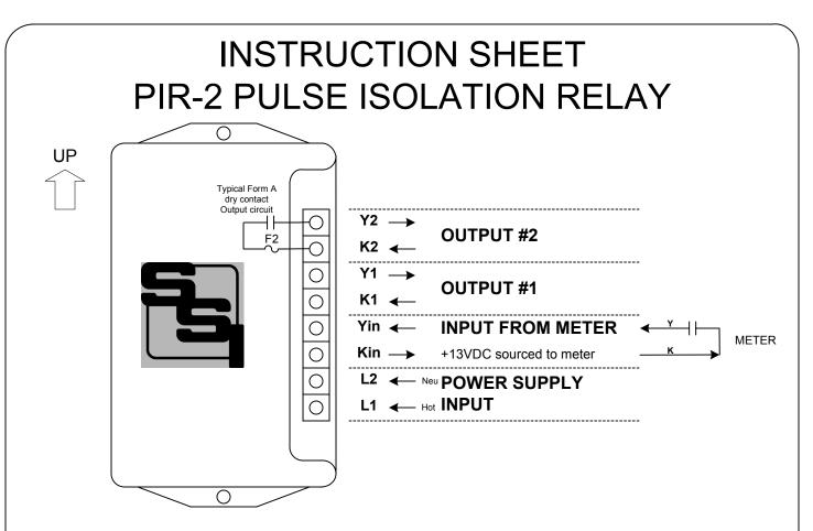
**MOUNTING POSITION -** Because the PIR-2 contains mercury-wetted relays, it must be mounted in a vertical position to operate correctly.
