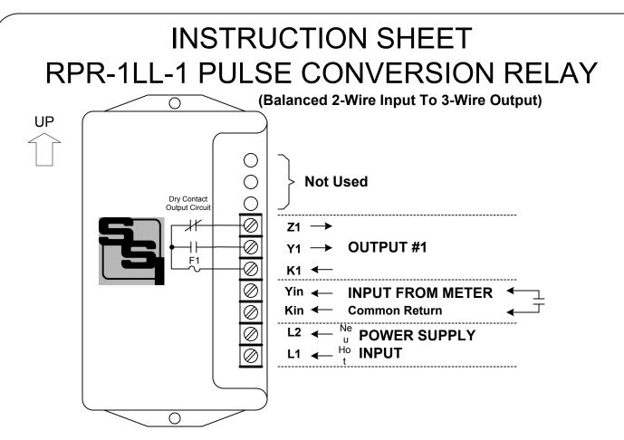
**MOUNTING POSITION -** Because the RPR-1LL-1 contains a mercury-wetted relay, it must be mounted in a vertical position to operate correctly.
