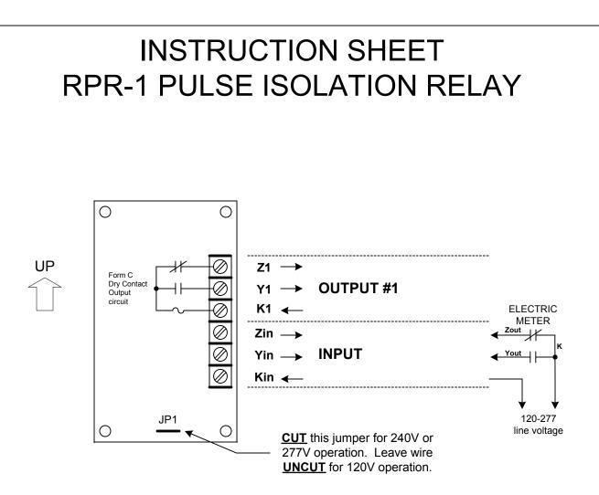
**MOUNTING POSITION -** Because the RPR-1 contains a mercury-wetted relay, it must be mounted in a vertical position to operate correctly.
