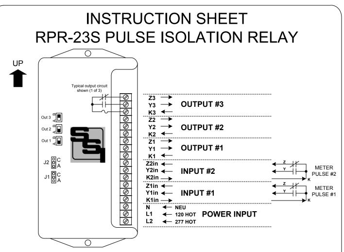
**MOUNTING POSITION -** Because the RPR-23S contains mercury-wetted relays, it must be mounted in a <u>vertical</u> position (as shown) to operate correctly. Note "UP" arrow above.
