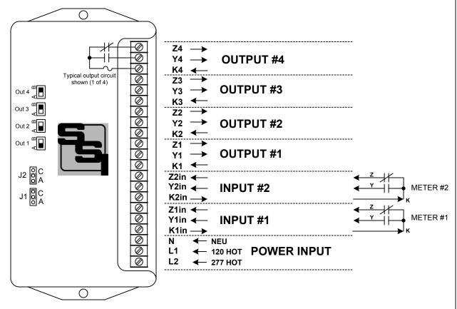
**MOUNTING POSITION -** Because the RPR-24S contains mercury-wetted relays, it must be mounted in a <u>vertical</u> position (as shown) to operate correctly.
