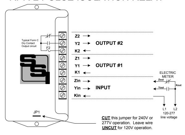
**MOUNTING POSITION -** Because the RPR-2 contains mercury-wetted relays, it must be mounted in a vertical position to operate correctly.
