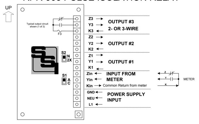
**MOUNTING POSITION -** Because the RPR-903 contains mercury-wetted relays, it must be mounted in a vertical position to operate correctly. The RPR-903 must be mounted in a suitable enclosure for the application.
